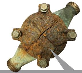
An improperly insulated water meter can result in a cracked meter in residences where the water meter is located in an unheated area.
