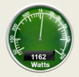
This green utility meter reading indicates that there is a surplus of energy being produced. When the meter turns red the house is using more energy than it is producing. The blue power production meter shows the electricity produced by the PV panels on the roof.
